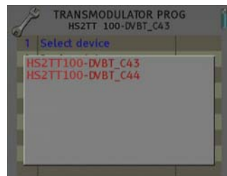
Interconnection of several modules, you can select which module you wish to program.
